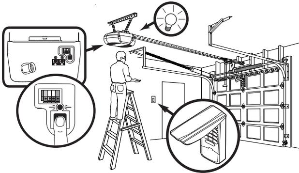
1. Press and release the "learn" button on motor unit. The learn indicator light will glow steadily for 30 seconds.
