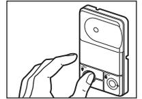
3. Continue holding both buttons while you press the push bar on the Premium Control Console (all three buttons are held).
