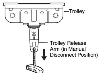
The *lockout feature* prevents the trolley from reconnecting automatically, and the door can be raised and lowered manually as often as necessary.
