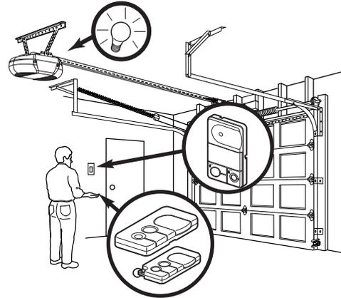
1. Press and release the “learn” button on the motor unit. The learn indicator light will glow steadily for 30 seconds.
