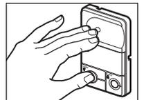
4. Release buttons when the motor unit lights blink. It has learned the code. If light bulbs are not installed, two clicks will be heard.
